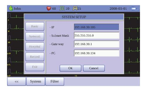
When selecting one of the 'IP', 'Subnet Mask', 'Gate Way' or 'PC', the keypad will show up. Then, input the information required and press OK button to save or ESC to cancel the information.
