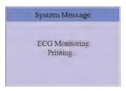
Press the 'ESC' key to stop the printing. Then, the message will be shown for a second as below and print out the paper until dotted line and the ECG Main page will show up.
