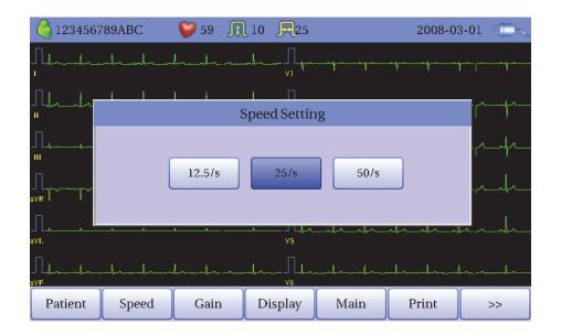
In order to adjust the speed of the ECG waveform, press the rotary key at the 'Speed' menu, then the mode will change to the information modification mode. Then, you can select the speed you want by clicking the rotary key.
